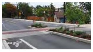
refuge island allows people to wait for vehicle traffic to dissipate from a protected gap in the median.
