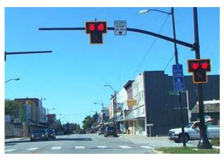
to illuminate. The pedestrian signal then indicates it is safe for the pedestrian to cross. HAWKs are typically more expensive than RRFBs and require power but are ideal to provide a safe crossing at heavily traveled pedestrian areas.
