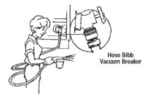
Residents are not allowed to immerse any type of hose or faucet fixture that is attached to the home's plumbing unless it has its own backflow prevention device.
