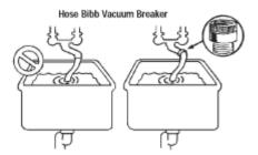
prevention devices on lawn irrigation systems. They must also provide proof that the backflow prevention device has been inspected by a certified tester. Most lawn irrigation installers and local plumbers can provide these services.
